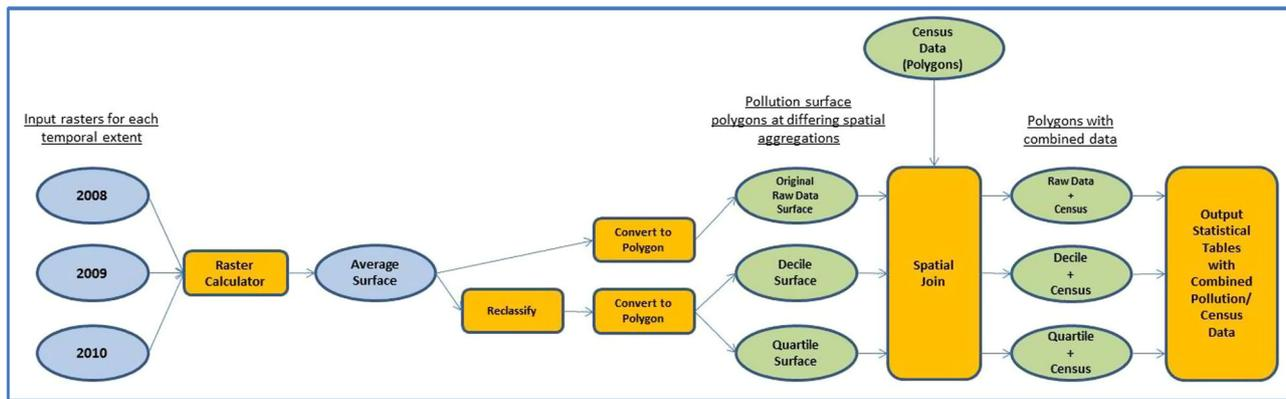
**Fig. 4** The model used to generate spatial files combining pollution surface data and census data. Ovals represent map data files, either rasters (blue) or polygons (green). Rectangles represent tools or
