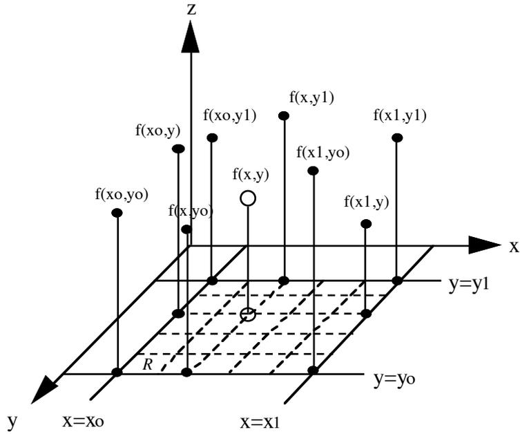
Figure 1. Schematic presentation of the two-dimensional net function interpolation. The  $z$  value of any internal net point  $(x,y)$  is estimated from the eight  $z$  values along the boundary of the region,  $R$ .
