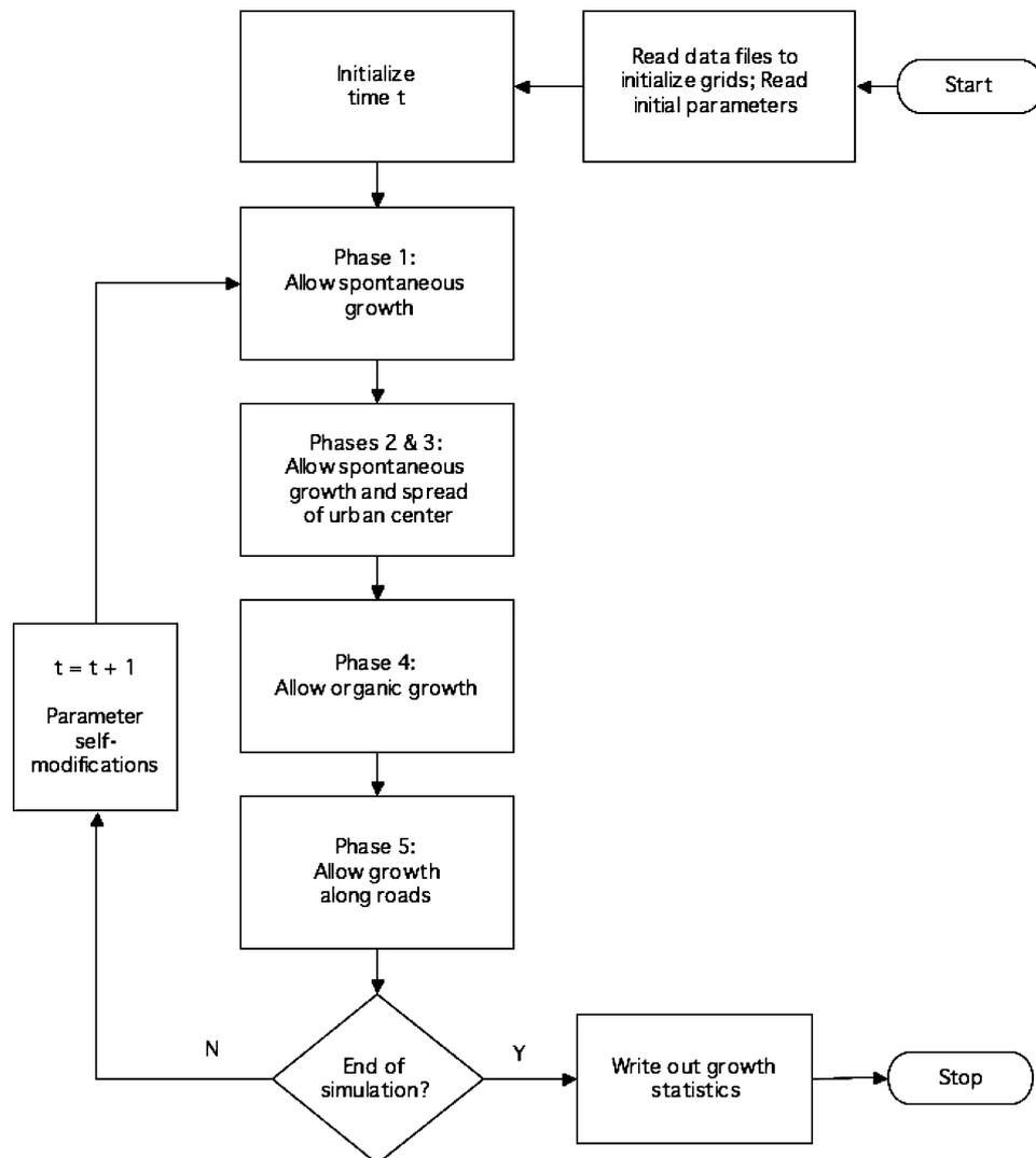
Figure 1. Flowchart of the HILT model, showing the five phases through which urbanization is simulated (based on the descriptions in Clarke *et al.* (1997)).
