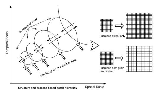
Fig. 3. Illustration of hierarchical scaling or extrapolating information along a hierarchical scaling ladder. Scaling up or down can be implemented by changing model grain size and extent successively across domains of scale.
