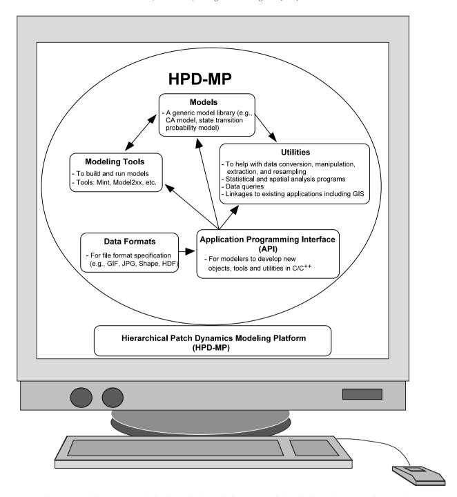
Fig. 6. Illustration of the structure of the hierarchical patch dynamics modeling platform (HPD-MP), showing the major components and their relationship.
