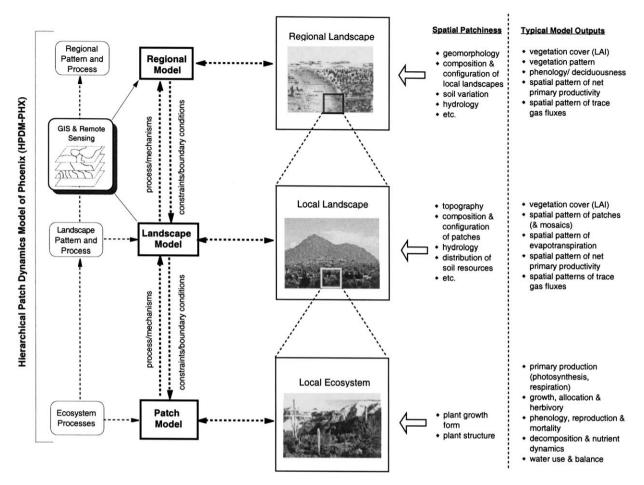
Fig. 5. Diagrammatic representation of the basic structure of the hierarchical patch dynamics model of the Phoenix urban landscape (HPD-PHX).
