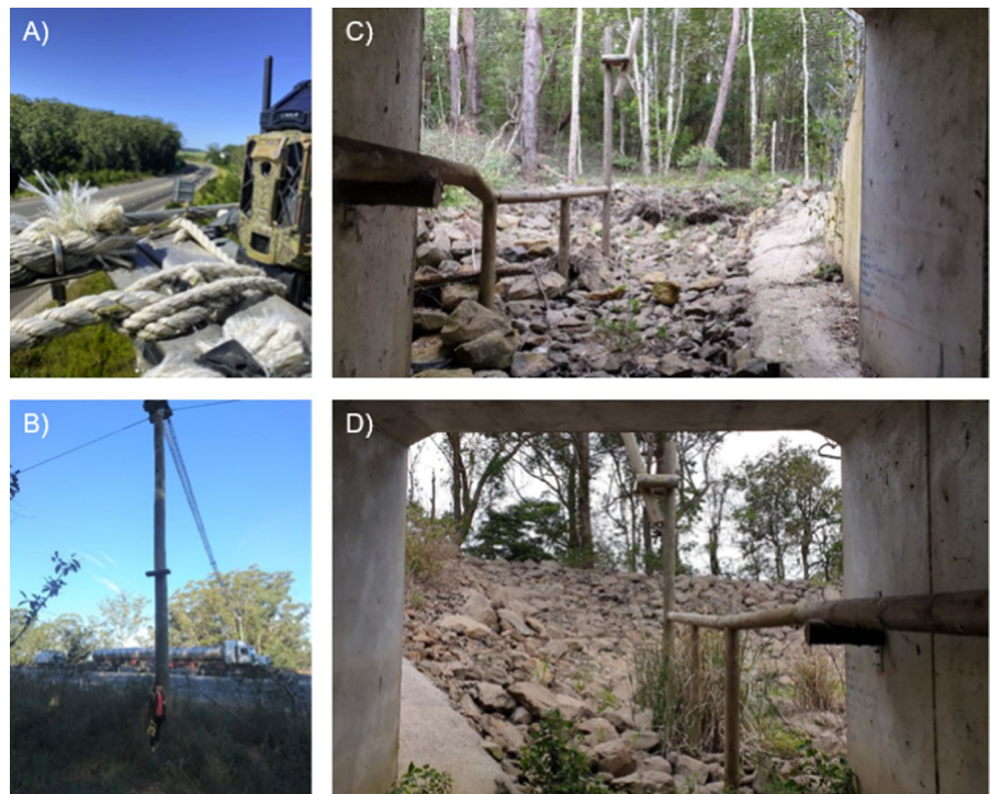
Fig. 3 Motion sensor cameras (A) used to monitor usage of the rope bridges (B) to cross over the Princes Highway. Cameras were also installed to monitor underpass tunnels and wooden bridges inside (C, D)
