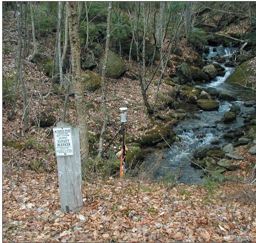
Figure 6. This location (BM1765 in Figure 5) offers a real challenge for GPS surveying. The marker is about 2 m below the adjacent road, under the forest canopy, in hilly terrain.
