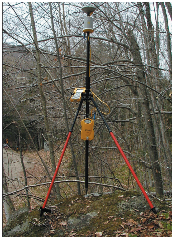
Figure 2. A rover antenna set up for differential GPS. The GPS antenna is the white disk at the top of the black pole; the receiver (yellow) is mounted halfway up the pole, facing the reader. The hand-held controller/data-logger (also yellow), used to set the data acquisition conditions and to download data after collection is complete, is mounted above the receiver.
